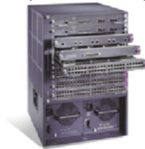
Figure 3 - Cisco 6509 Catalyst Switching Chassis
